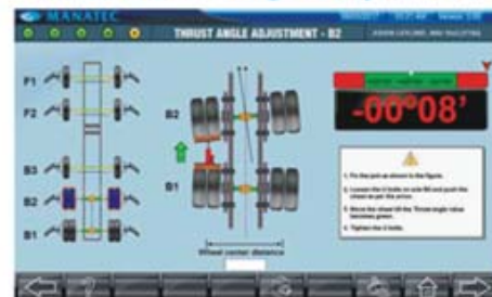
Alignment of Rear multi axles
