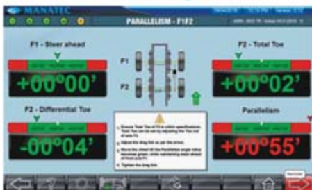
Alignment of Front twin steerable axles
